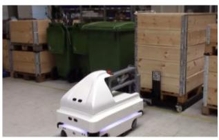
Utilized to tow carts within a facility. Servo operated hook allows for docking and un-docking of carts for transport. Tow up to 1,100 lbs.
