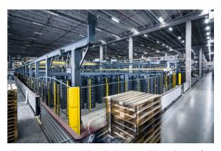
Cimcorp's Layer Pick solution combines large, fast gantry robots with a clamp gripper and vacuum picking head for order picking. Using varying force and vacuum strength based on the SKU to be handled, the system can pick virtually any consumer product on the market.
