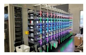
Pick-to-light systems are simple, but robust systems designed to streamline picking operations, therefore increasing efficiency, productivity and accuracy while reducing costs.
