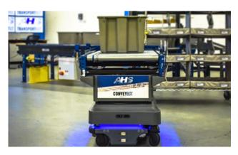
Allows for cases, totes or other materials to be conveyed onto or off of a MiR robot. Will dynamically replace fixed conveyor solutions or utilized for sortation.
