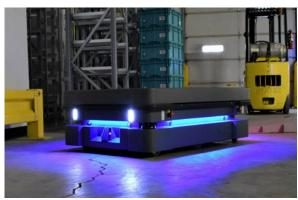
This is MiR's most powerful robot, designed to automate and optimize the internal transportation of heavy payloads and pallets, with a payload capacity of 1000 kg or 2200 pounds.
