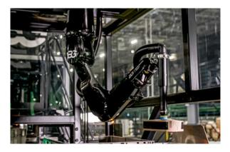
Berkshire Grey's piece picking robots feature industrial robotic arms with smooth and natural 6-DOF optimized motions for maximum efficiency.
