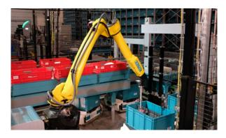
The Skypicker is a fully automated warehouse picking module that completes the Skypod order preparation solution. It is equipped with an articulated arm and order mover that allows simultaneous preparation of four orders.
