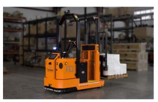
The Max N10 Pallet Stacker is an automated counterbalanced lift truck with a payload capacity of 1,770 lbs, and a high capacity version for up to 2,650 lbs.
