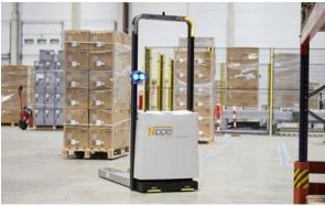
The Nipper is a compact automated vehicle for unmanned, internal pallet transport. It can easily lift pallets up to 1000kg and safely navigate through narrow spaces.
