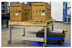
Utilized to move carts of all sizes or up to 900lbs. Allows operators to focus on value added operations instead of moving carts/pallets from position to position.
