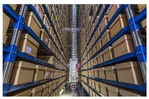
An Automated Storage and Retrieval System (AS/RS) is a combination of equipment and controls that handle, store and retrieve materials as needed with precision, accuracy, and speed.
